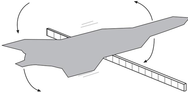
If your center of mass is in front of the center of pressure, your rocket should be stable. Proceed to the swing test. If the two centers are next to or on top of each other, add more clay to the nosecone of the rocket. This will move the center of mass forward. Repeat steps 2 and 3 and then proceed to the swing test.
