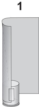
**Wrap and tape a tube of paper around the film canister. The lid end of the canister goes down!**
