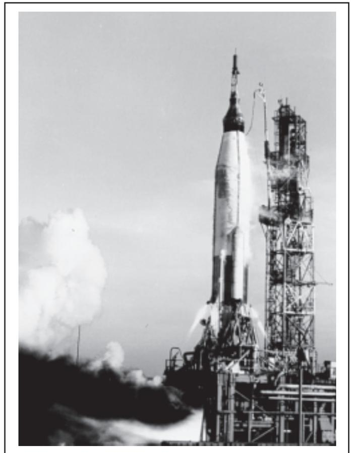
An Atlas launch vehicle, with a *Mercury* space capsule at the top, underwent a static firing test to verify engine systems before its actual launch. The *Mercury/Atlas* combination launched four *Mercury* orbital missions including the historic first American orbital flight of John Glenn.
