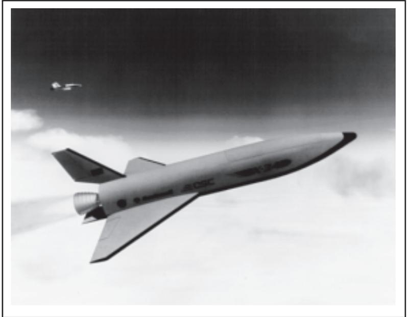
NASA has chosen this concept to replace the Space Shuttle fleet in the 21st century. The X-33 will be a single-stage-to-orbit vehicle in which the entire vehicle lifts off into space and returns to Earth intact.
