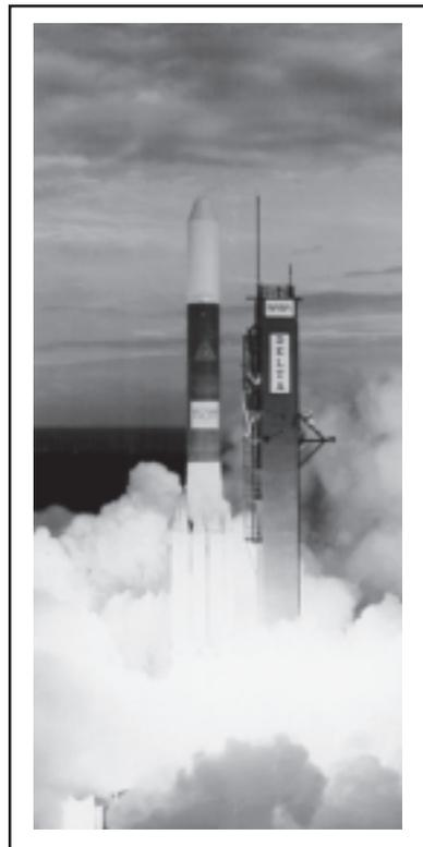
One of NASA's most successful rockets is the Delta. The Delta can be configured in a variety of ways to change its performance to meet needs of the mission. It is capable of carrying over 5,000 kilograms to a 185 kilometer high orbit or 1,180 kilograms to a geosynchronous orbit with an attached booster stage. This Delta lifted the *Galaxy-C* communication satellite to space on September 21, 1984.
