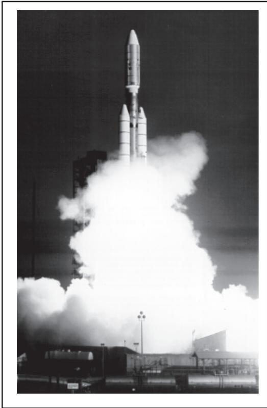
A Titan III Centaur rocket carried *Voyager 1*, the first interplanetary spacecraft to fly by both Jupiter and Saturn, into space on September 5, 1975. The Titan, a U.S. Air Force missile, combined with NASA's Centaur upper stage and two additional side-mounted boosters, provided the needed thrust to launch *Voyager*.
