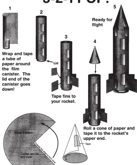
1. Wrap and tape a tube of paper around the film canister. The lid end of the canister goes down!
