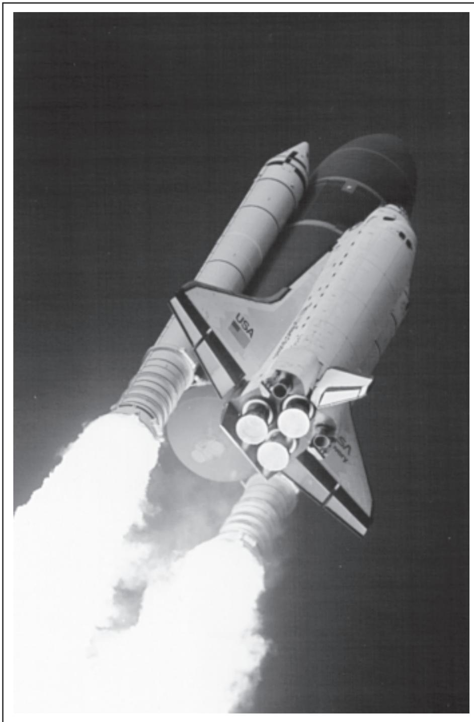
Today, NASA Astronauts launch into space onboard the Space Shuttle. The Shuttle consists of a winged orbiter that climbs into space as a rocket, orbits Earth as a satellite, and lands on a runway as an airplane. Two recoverable solid rocket boosters provide additional thrust and an expendable external tank carries the propellants for the orbiter's main engines. This was the launch of STS-53 on December 2, 1992.
