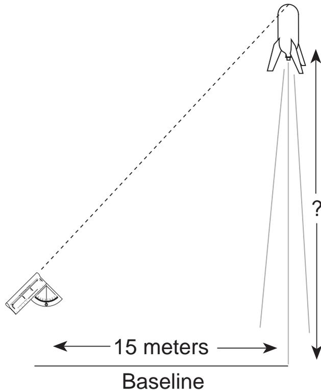
rocket, the tracking station should be 5, 15, or 30 meters away. (Generally, a 5-meter distance is sufficient for paper rockets and antacid-power rockets. A 15-meter distance is sufficient for bottle rockets, and a 30-meter distance is sufficient for model rockets.
