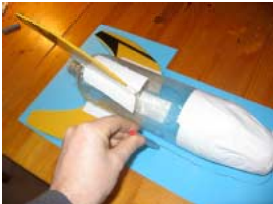
Illustration of the silhouette technique for estimating the centre of pressure.
