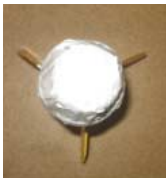
Left: A photograph of the ‘Flying Gherkin’ from directly above its nose cone: this is what you would see if the rocket were flying directly towards you.
