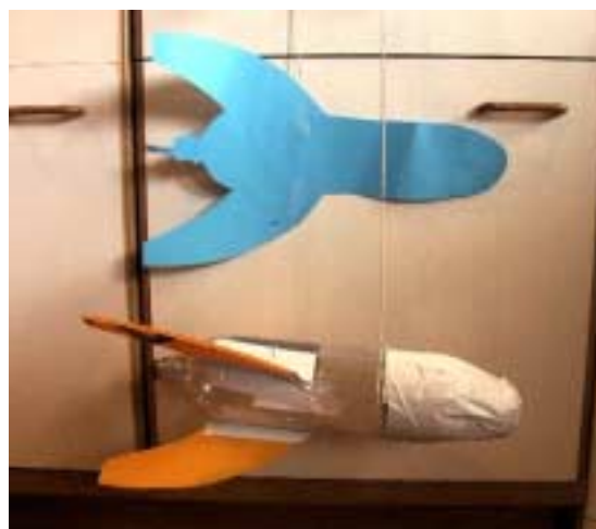
Illustration of the silhouette technique for estimating the centre of pressure.
